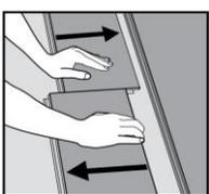
**Disassembling** Your floor can very easy be disassembled, which enables replacement during installation and also during use. Separate the whole row by carefully lifting up and slightly knocking just above the joint. Fold up or angle and release the whole long side. Disassemble the panels by sliding horizontally where possible or fold up and angle to release.
