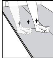
**Figs 8c** As it flattens itself to the floor press or gently tap the top of the short end of the installed panel until its flat. Finish installing this plank by tapping it with a tapping block on the long side to ensure secure installation. **Make sure long edge and short ends are flush, no gaps.**
